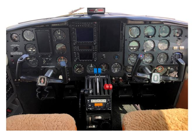
MFD Bendix 500 Multi-Function Display Aspen EFD 1000C3 Pro PDF Auto Pilot Bendix KN1530 Garmin GNS 530W Garmin GNS 430W GTX 345 & 335 TPX GMA 345 Audio Weather Radar Bendix RDR 250 HP GDL 69 GDL88 ADS-B Transceiver
