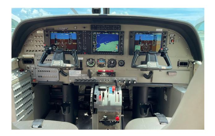
Flight System Garmin G1000 **DME** Honeywell KN-63 **ADF** Autopilot Garmin G1000 Honeywell KR-87 Radar Garmin GWX-70 Transponders **Dual Garmin GTX-33** Dual Garmin GIA-63W Traffic Garmin GTS-825 Comms **Dual Garmin GIA-63W** Terrain Navs Garmin (TAWS-B)
