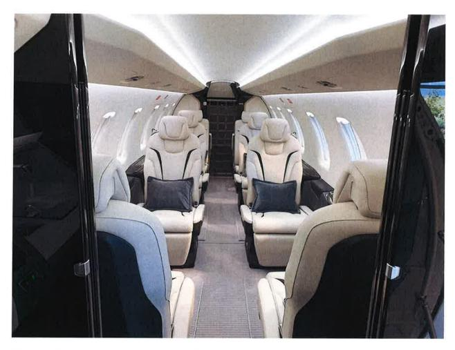
The eight (8) passenger interior features six (6) executive and two (2) commuter type seats. There is also a forward private lavatory. Ample storage space is located in various cabinets in the main cabin as well as inflight access to the extra-large rear cargo area with exterior top-hinged cargo door.
